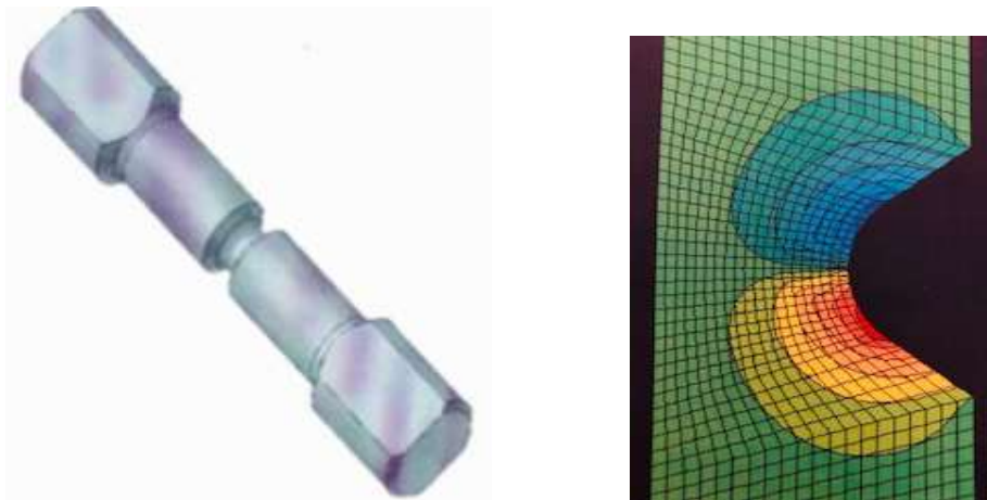
Fig. 2 3D view and the finite element model (a) 3D view of the specimen (b) Abacus model
